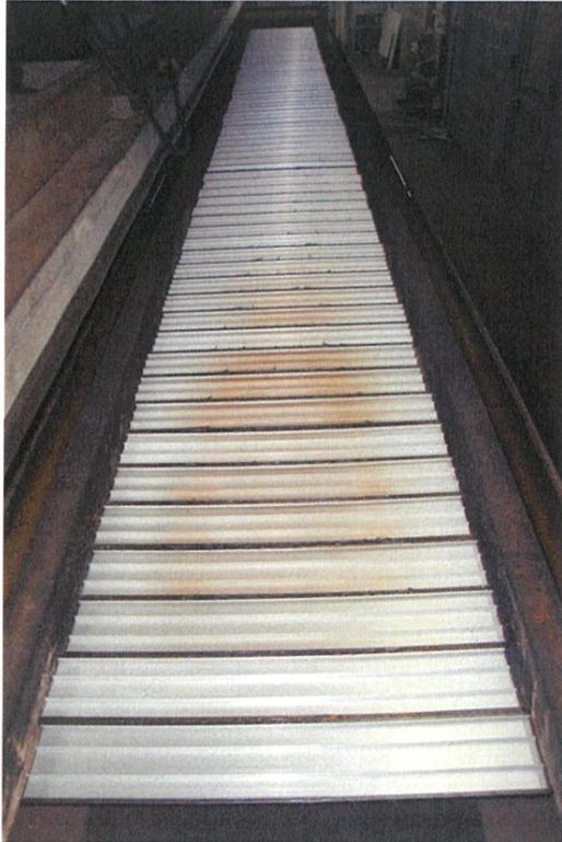
After testing (unexposed side,near side of burner)
